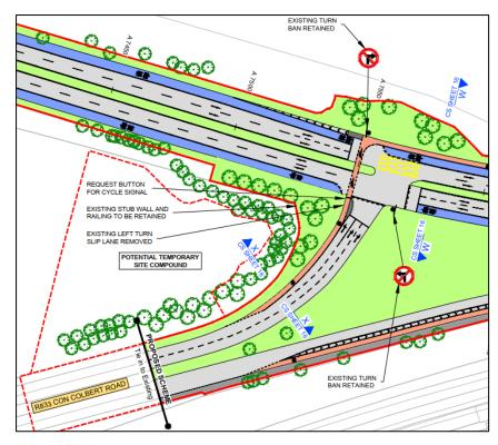
Figure 3-1 Preliminary Design of the Proposed Scheme Tie-in with the Existing Layout
